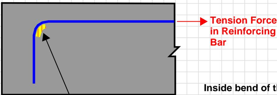
Inside bend of the reinforcing bar bears onto the concrete. If this bearing area is small (tight bend as shown) we can locally crush the concrete
