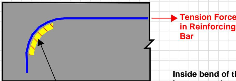
Inside bend of the reinforcing bar bears onto the concrete. The bar in this sketch has a larger bend radius and therefore the bearing area is larger. There is less chance of crushing the concrete in this example
