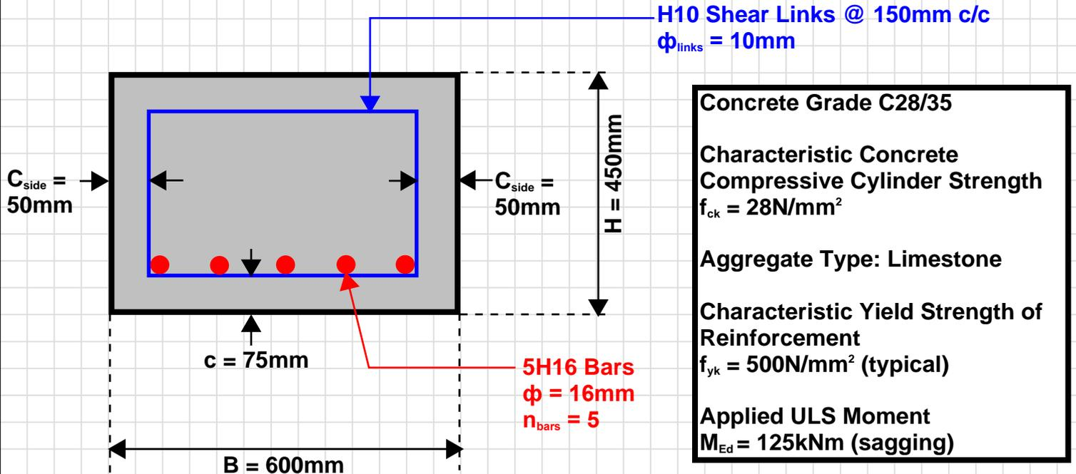
**Tensile Design of RC Beam**
