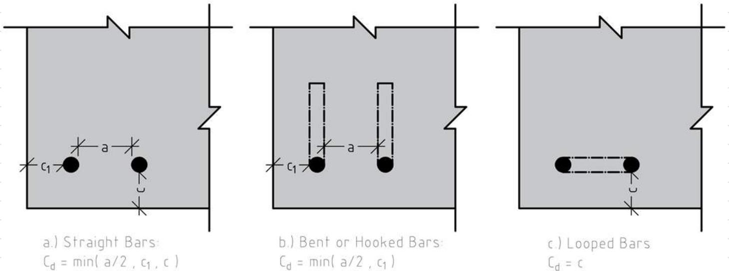
We have straight bars in a beam which is the case on the far left of the diagram above
