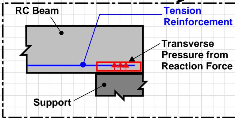
In our example lets assume a dead bearing support similar to that shown in the diagram above. Lets take an applied transverse ULS pressure of  $p = 5\text{N/mm}^2$
