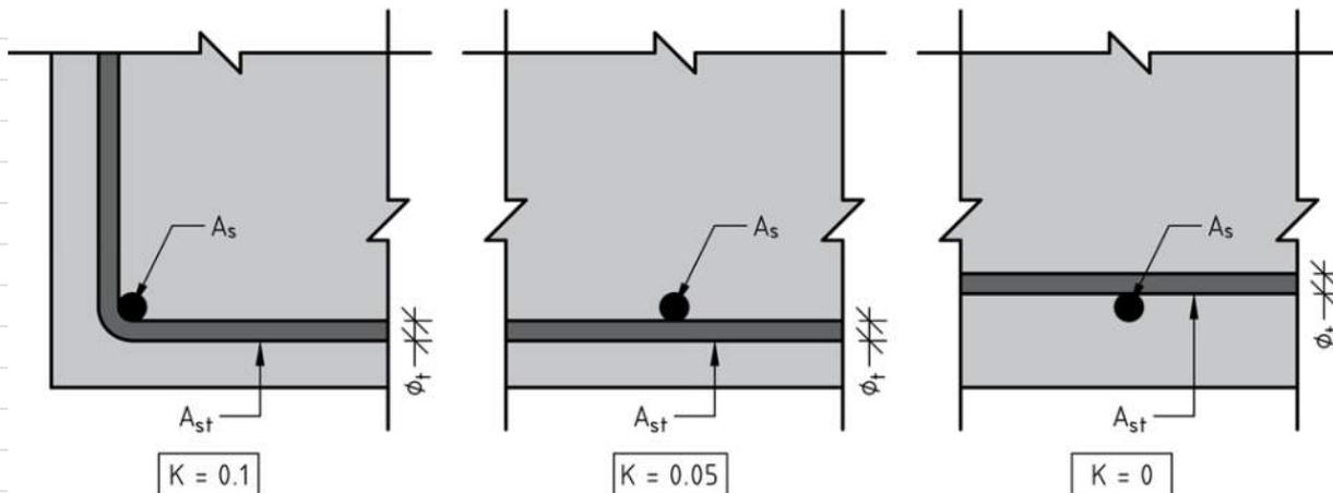
$A_s$  = The reinforcement we're trying to anchor (i.e. applied tension/compression force is in and out of the page)
